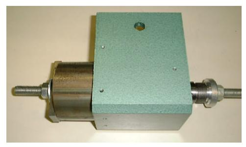
• If you don't have the R8 Spindle Installation Kit, put the 3-1/2" hex electrical box on the bottom end as shown below. Put a 1/2" flat washer or two on behind the electrical box, followed by a 1/2" nut. If your bearings are particularly tight in the spindle housing you might need to add a stiffener behind the electrical box to keep from crushing it. A piece of angle iron drilled for the threaded rod works fine.
